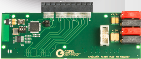
ChipVORX-I/O module with test adapters for PCIe x8 plugin cards
