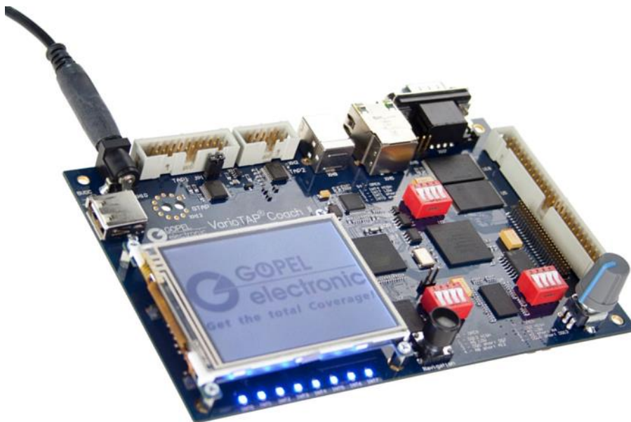
Figure 3-1 PCB with multiple BScan devices, memory types and interfaces
