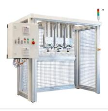
The seat occupancy is checked by simulating various occupancy states. Depending on the type of ODS, the simulation can be performed by applying a force or by capacitive influence of the electrical field.
