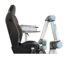
Many monotonous, recurring, manual activities can be completed with a cobot to significantly increase the degree of automation. Coby complements the OsCAR test system and can also be integrated into test systems from other suppliers.
