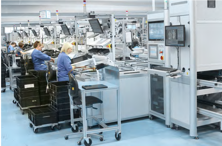
Production line with manual loading and final optical inspection.
