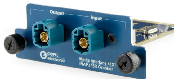
Figure 2-9: INAP375R Top board
