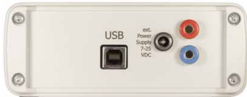
Figure 2-3: basicCON 4113 – rear side
