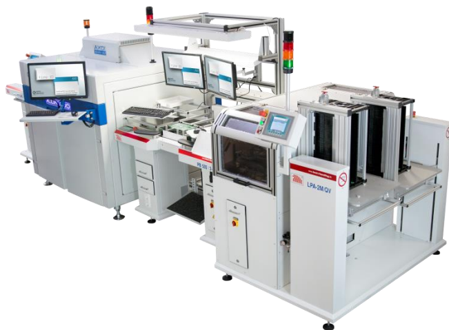
Fig. 1: Part of a production line with AXI system and inline verification station
