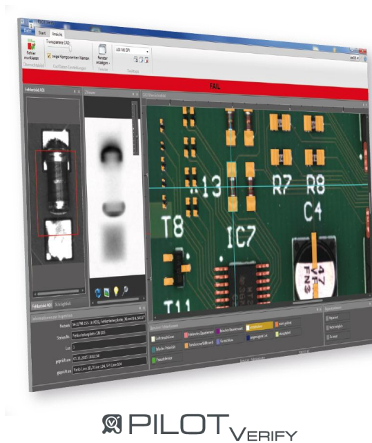
Fig. 2: Verification station software PILOT Verify with AOI and AXI fault images
