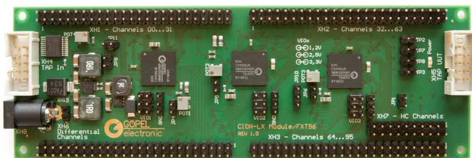
Figure 8: Multifunctional mixed-signal I/O module CION-LX/FXT96 with TAP cascading
