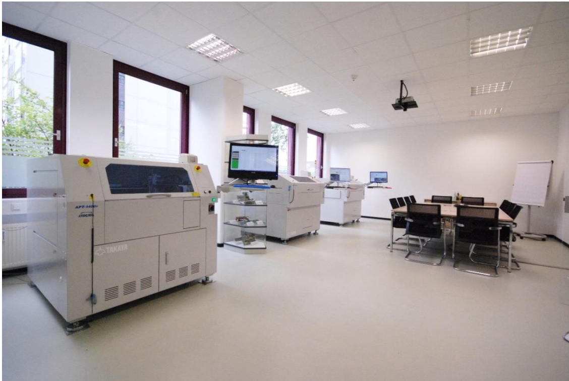
Image: Various Flying Probe Testers from TAKAYA at the site in Düsseldorf. Front: the flagship APT-1400F
