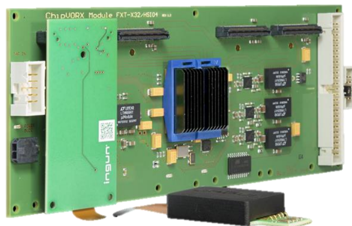
Figure 4: ChipVORX module for testing high-speed interfaces
