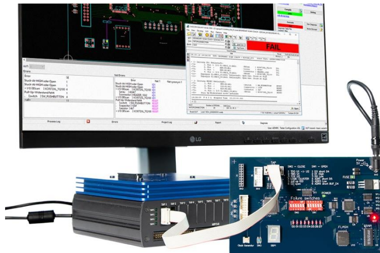
Figure 3: Embedded JTAG Solutions Controller "SCANFLEX II" in operation with SYSTEM CASCON software
