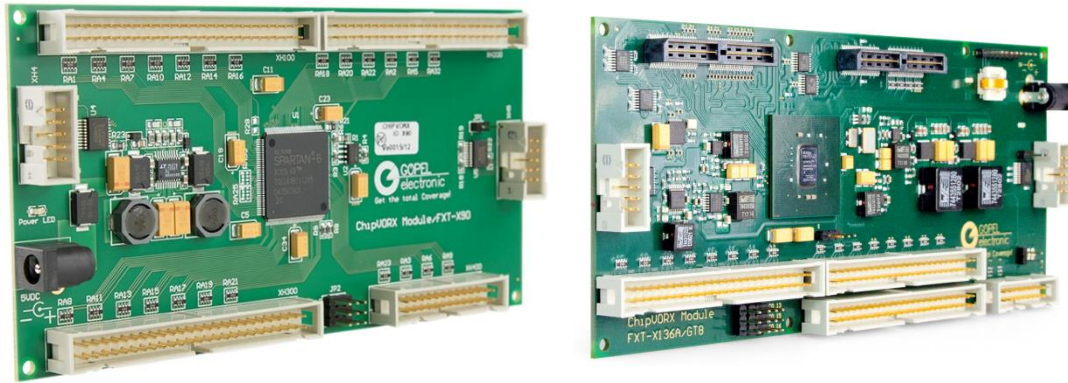
Figure 7: ChipVORX modules with integrated FPGA
