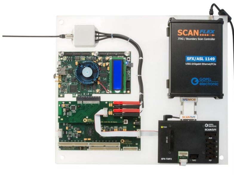
Graphic 7: Test set-up with CION LX-Board, SCANFLEX-Controller and PCIe-Adapter
