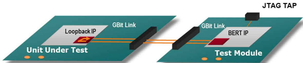
Graphic 6: Loopback test with adapter board
