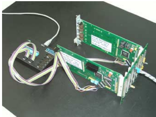
Image4: Test set-up with a small board and two Boundary Scan paths
