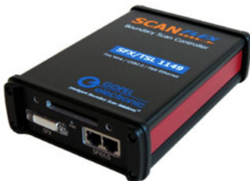
Bild 3: Hardware – Boundary Scan Controller von GÖPEL electronic (SFX-TSL1149.x)
