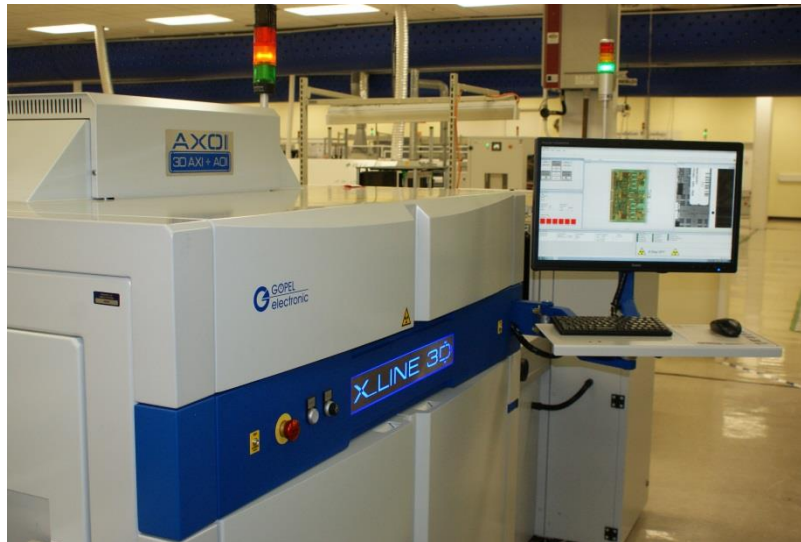
Figure 2 – X Line 3D X-ray inspection system in production (source: Foundation Technology)
