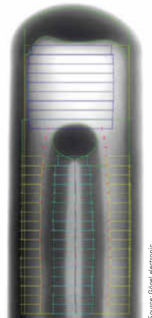
Inspection of the sensor tip. Among other things, distances, thicknesses, and the welding of two wires are checked
