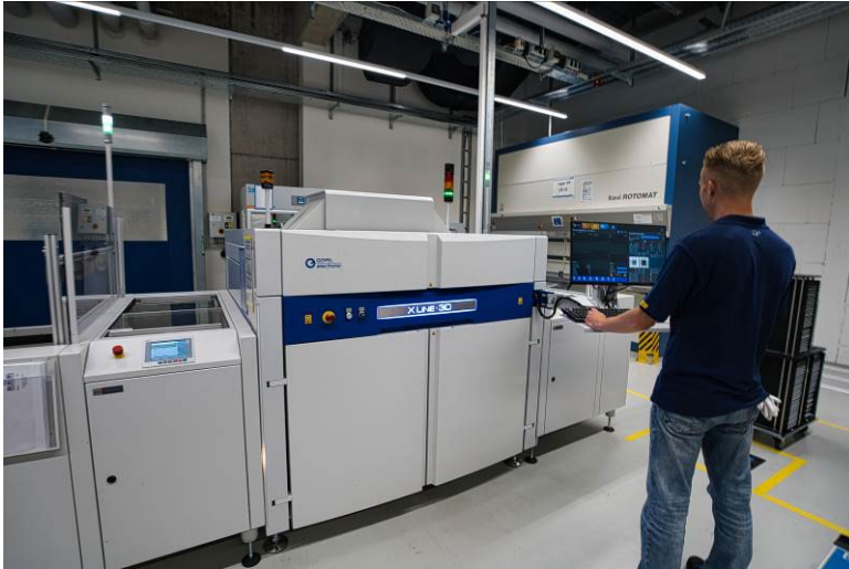
Figure 2: X-Line from GÖPEL electronic for X-ray inspection (Source: Hekatron Manufacturing GmbH)
