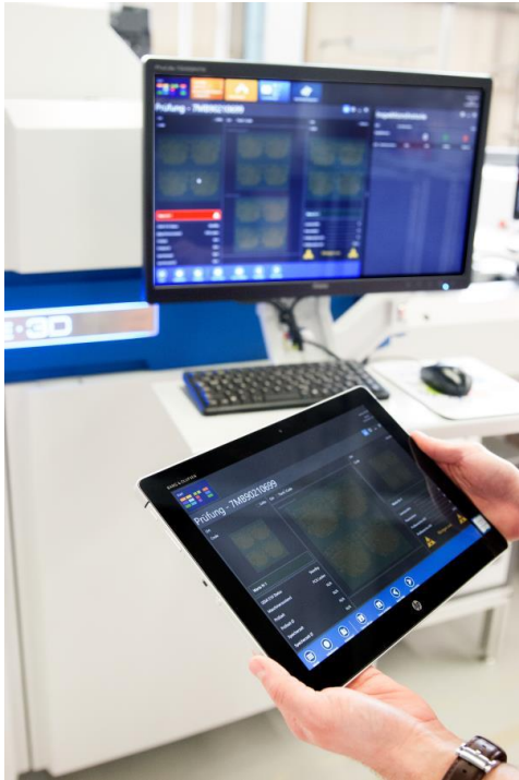
Figure 7: Monitoring and controlling the X-ray system in a smart factory from a tablet
