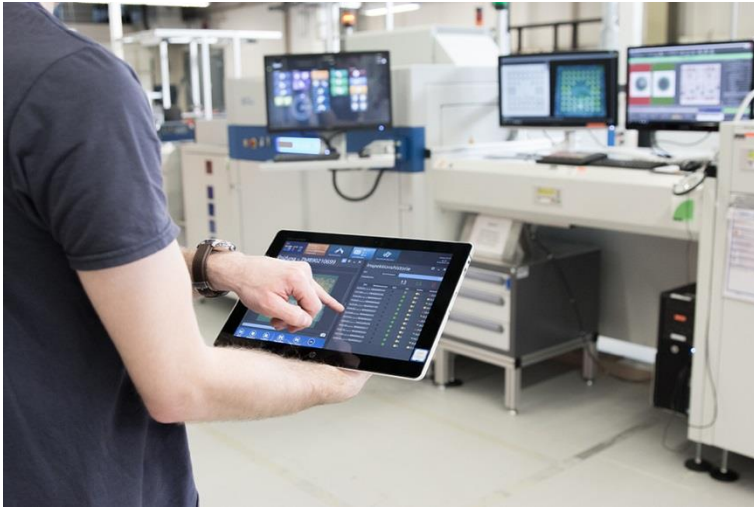
Fig. 3: Monitoring and controlling the X-ray system from a tablet
