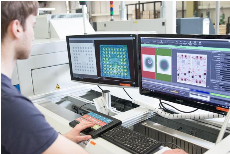
Fig. 1: Verification station for viewing detected faults: BGA with void
