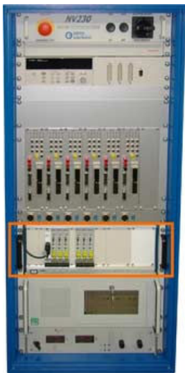
Image 3: MOST PXI test system
