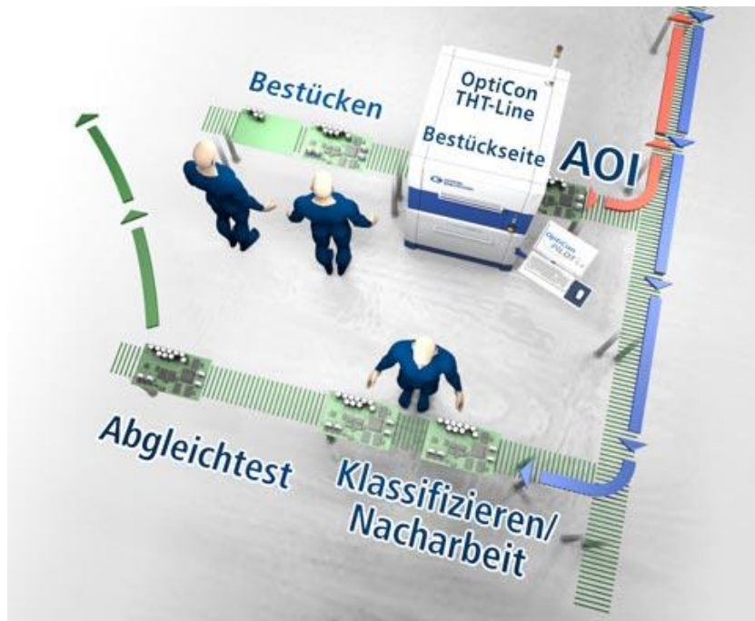
Image 3: Diagram of assembly and reworking station
