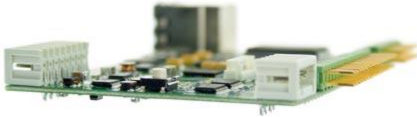
Image3: SMD assembly with several THT components
