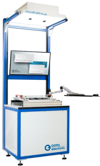
Figure 1: AOI module for component inspection at the assembly workstation
