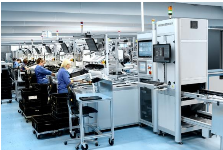
Fig. 1: The THT manual assembly stations, left, and the downstream inspection system MultiCam Line, right
