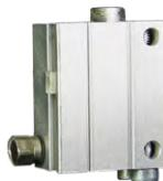
Pneumatic cylinder for automatically opening the cover once the test procedure is finished. (This option serves exclusively for opening the cover and cannot be retrofitted.)
