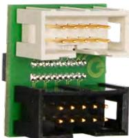
Adapter from a 20-pin high-density socket to two 10-pin low-density plug connectors
