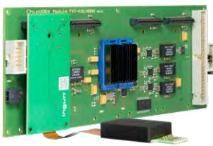
ChipVORX module for testing high-speed interfaces
