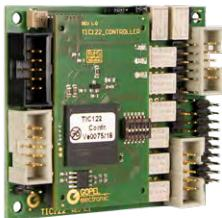
TAP Interface Card as a fixture assembly module for connection to replaceable or built-in TEM or TEM / ISO
