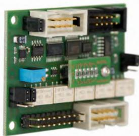
TAP Interface Card as a fixture assembly module in a climatic chamber for connection to replaceable or built-in TEM or TEM/ISO
