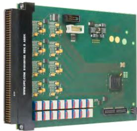
Fixture SCANFLEX digital I/O module for gang applications
