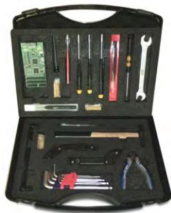
Tool kit for JULIET, including CION module and wearing parts package.
