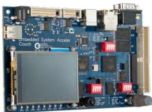
Complex "Embedded System Access (ESA)" training board for JTAG / Boundary Scan, VarioTAP and ChipVORX applications
