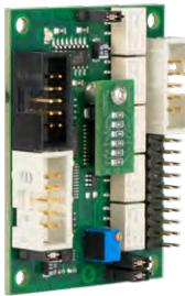
TAP Interface Card as a fixture assembly module for connection to replaceable or built-in TEM or TEM/ISO
